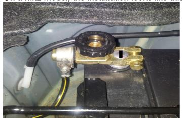
Once the battery disconnect switch is fitted, the battery can be connected by turning the black knob clockwise, and disconnected by turning it anti-clockwise.
